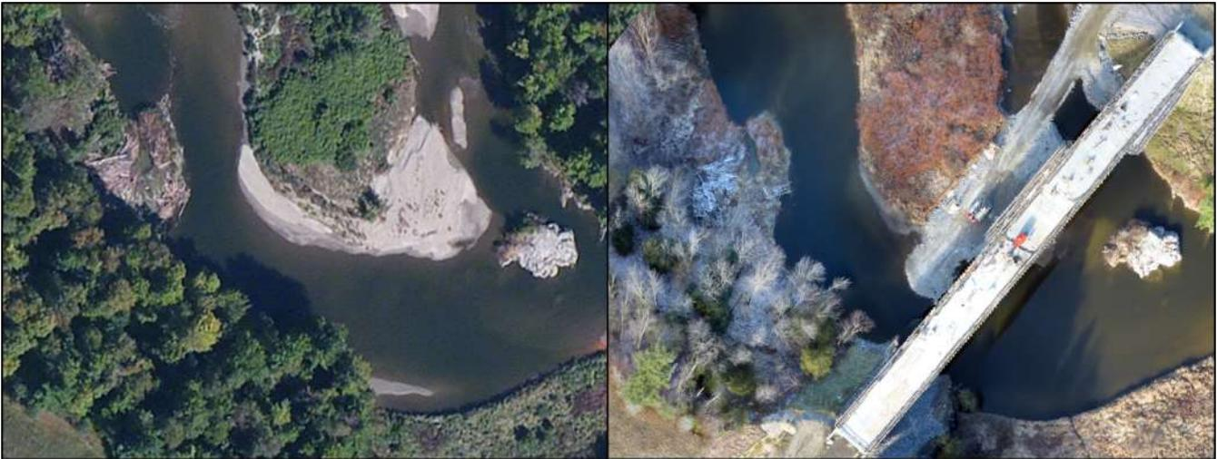
*Figure 7. Imagery from a new road construction project. The pre-construction imagery (left) was acquired by a manned aerial system as part of a statewide mapping project. The imagery acquired during construction (right) was done by a lightweight UAS during RITARS-12-H-UVM.*
