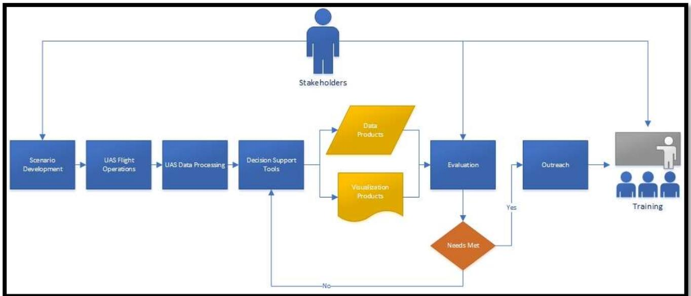
Figure 2. Generalized workflow for UAS operations.
