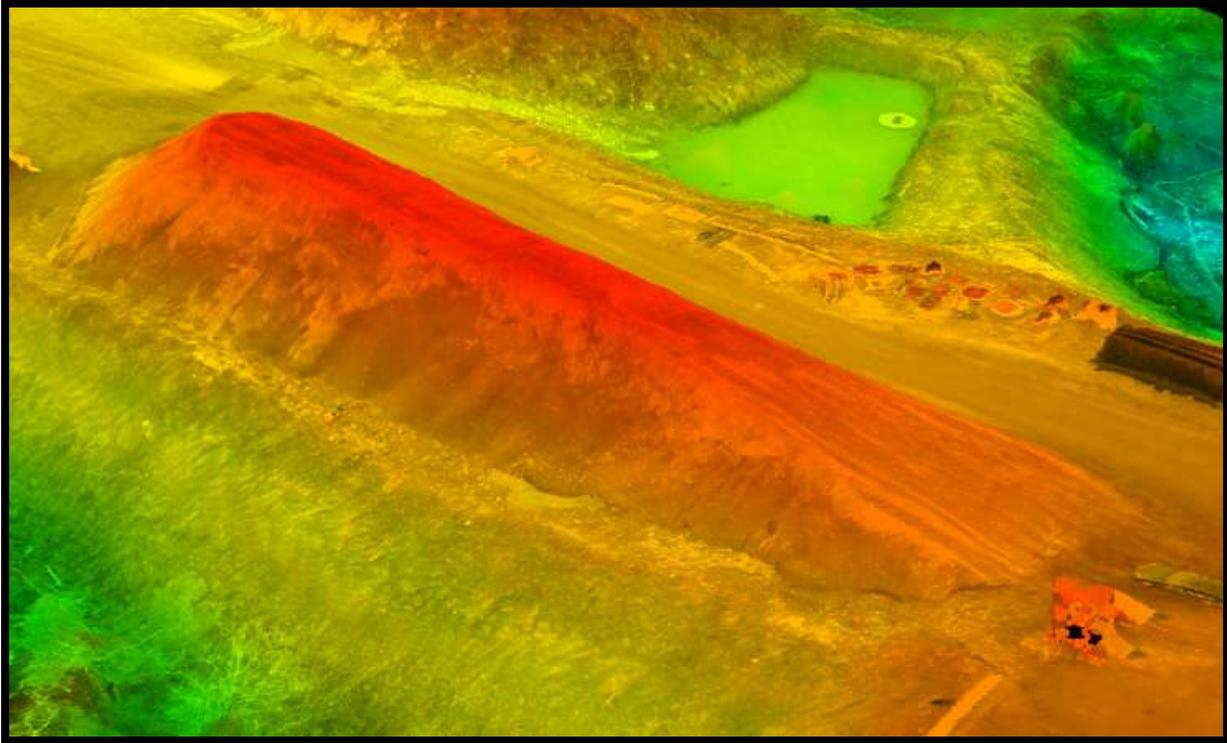
*Figure 1. 3D visualization of spoil pile for a transportation construction site generated from UAS imagery collected during our current RITA-12-H-UVM.*
