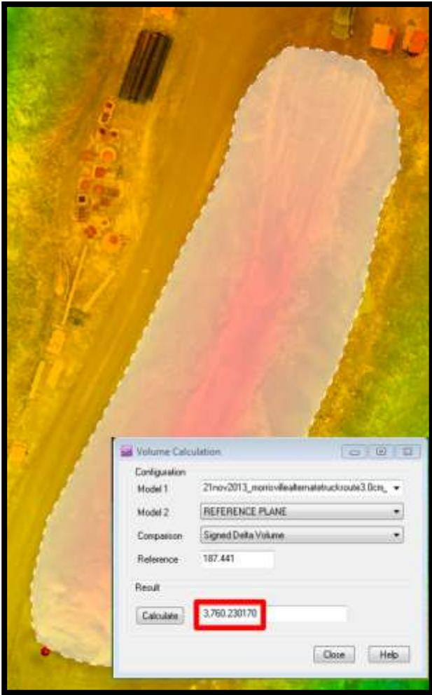
Figure 5. As part of our current RITA project, we have developed decision support tools using commercial software, such as Applied Imagery's Quick Terrain Modeler. This example shows how volumetric information can be extracted from 3D data acquired by a UAS. Applied Imagery is a project partner for this proposed supplemental grant.
